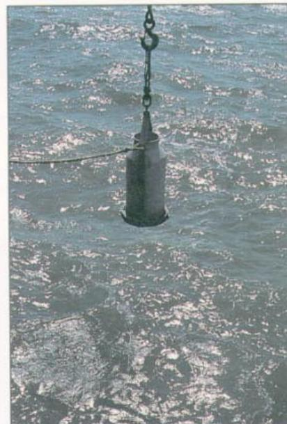
Plate 9. Surface water sampler (40 l churn)
