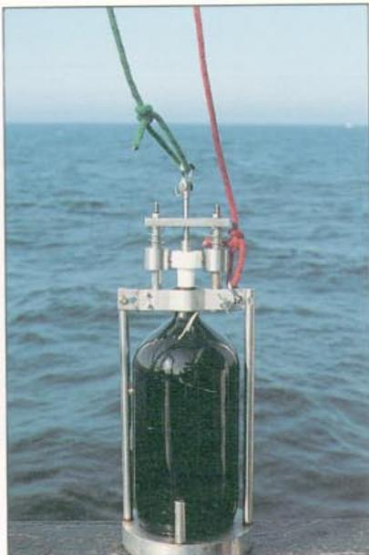
Plate 8. Surface water sampler (2.5 l)
