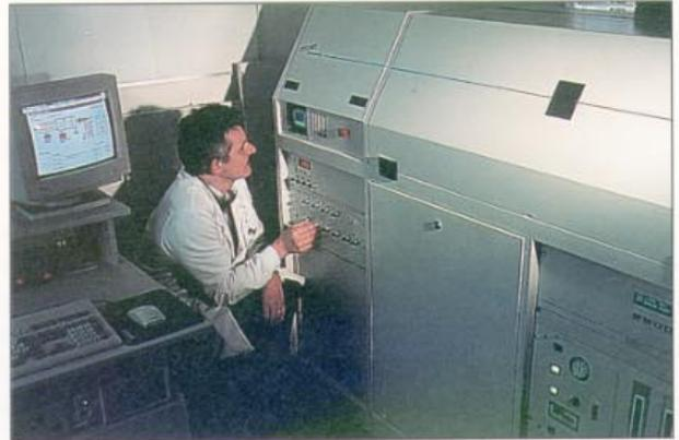
Plate 11. Inductively-coupled plasma/mass spectrometer
