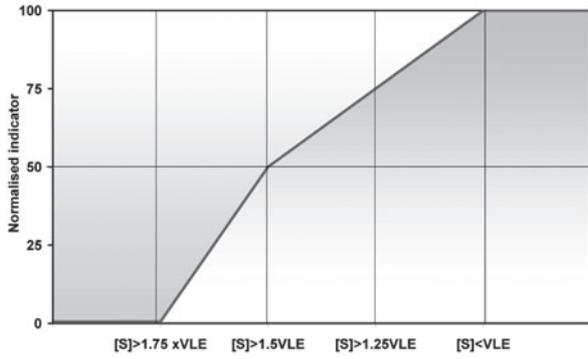
Fig. 3. Penalty curve for the determination of the pressure indicator of compliance with emission limits.
