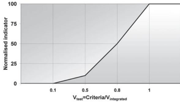
Fig. 4. General shape of a penalty curve to determine the normalized indicator.
